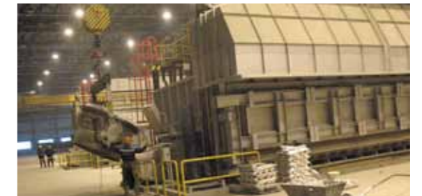
METAL POURING INTO THE MIXER, CASTHOUSE, IRKUTSK ALUMINIUM SMELTER
