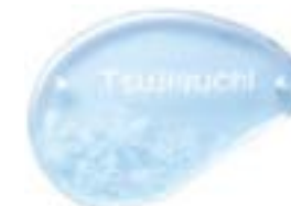
Glass plate made from recycled waste LCD panel glass (Photo courtesy of Minocraft Corporation)
