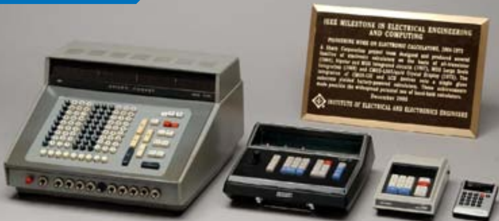
Commemorative plaque from the IEEE (in background) and Sharp electronic calculators recognized as an IEEE Milestone for innovations in size and power-consumption reduction (From left) CS-10A all-transistor-diode calculator, CS-16A IC calculator, QT-8D LSI calculator, and EL-805 LCD pocket calculator
