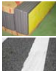
Scrap glass used effectively as an insulation material (top) and in reflective marking materials for lane stripes on roadways
