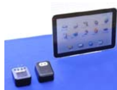
Intelligent power-measuring plugs (left) and media tablet
