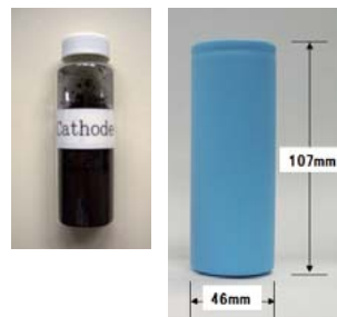
New manganese-based cathode material (left) Prototype battery cell (right)
