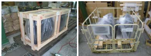
One-way wooden crates (left) replaced by collapsible, reusable crates (right)
